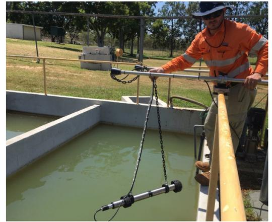
Xylem’s system and installation team member immersing the UV-VIS CarboVis 705 IQ multi-parameter six-in-one sensor with BOD and TSS measurement in the final chlorine contact tank.
