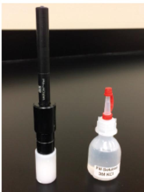
**Figure 8.** Contents of box that reference electrode ships in. The white cap threads on to the VARIION Ref and should be re-filled with 3M KCl Fill Solution for storage and shipment
