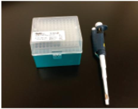
**Figure 7.** Typical pipette and tips used for colorimetric determination of ammonia, nitrate, potassium, and chloride)
