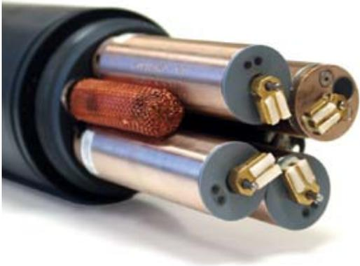
*YSI 6600 sonde with installed anti-fouling kit*
