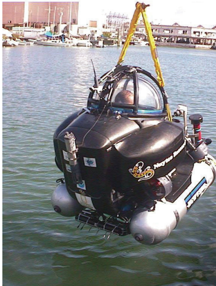
An SSE DeepWorker 2000 submersible vehicle with a YSI 6600 Multiparameter sonde.
